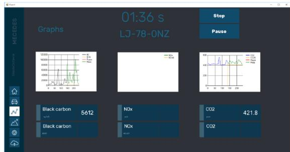
SPIDer™ application: during measurement Smart-EYE recognizes the license plate and retrieves relevant vehicle information (left). Real-time display of Black Carbon and CO2 concentration for emission factor determination.
